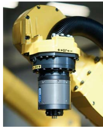
Tool changer TC20-ID enables tidy installations, free of loose cables that could inhibit robot movement.
